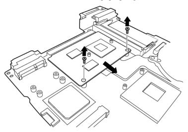
Figure 4-42 Removing screws securing VGA Card
